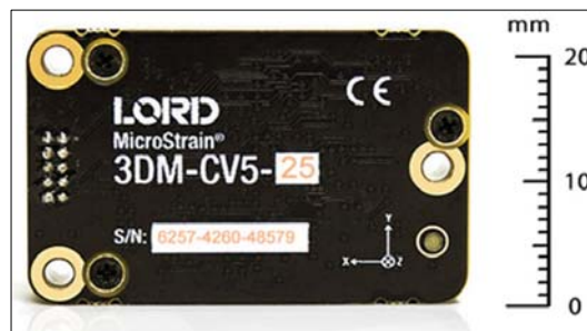
FIG 3.11 – Sensor LORD MicroStrain 3DM-CV5-25 (imagem de www.microstrain.com )
